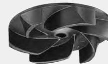
The vortex impeller is adopted in every series except for the PSF-series. Rotation of the impeller produces a whirling, centrifugal action between the impeller and the pump casing, and it moves the fluid through the pump. Being coupled with a wide pump casing, wastewater containing solid matters can be pumped out without obstruction.
