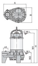
C.W.L.: Continuous Running Water Level L.W.L.: Lowest Running Water Level
