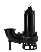
The B-series is a submersible channel impeller pump designed for handling raw sewage, wastewater and heavy-duty industrial applications, where the pump is subject to complete submersion and requires maximum reliability. The B-series has a proven track record for offering long life in both continuous and intermittent sump applications. It is available as an extended line-up from 50 to 800mm discharge bores.
