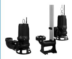
The B-series is a submersible channel impeller pump designed for handling raw sewage, wastewater and heavy-duty industrial applications, where the pump is subject to complete submersion and requires maximum reliability. The B-series has a proven track record for offering long life in both continuous and intermittent sump applications. It is available as an extended line-up from 50 to 800mm discharge bores.
