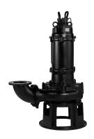
The B-series is a submersible channel impeller pump designed for handling raw sewage, wastewater and heavy-duty industrial applications, where the pump is subject to complete submersion and requires maximum reliability. The B-series has a proven track record for offering long life in both continuous and intermittent sump applications. It is available as an extended line-up from 50 to 800mm discharge bores.
