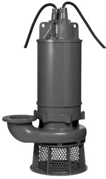
The GSZ-4-series is a submersible three-phase cast iron high head and high volume heavy-duty drainage pump driven by a 4-pole motor. The side discharge, spiral design allows smoother passage of the sucked solid matters. The motor is cooled by a water jacket that assures efficient motor cooling even when it operates with its motor exposed to air. The pump incorporates seal pressure relief ports that prevent the pumping pressure from applying to the shaft seal.
