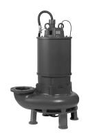
The GSZ-6-series is a submersible three-phase high power and high volume heavy-duty drainage pump driven by a 6-pole motor. In combination with abrasion-resistant wear parts, the very low speed motor ensures extremely long wear life. The side discharge, spiral design allows smoother passage of the sucked solid matters. The motor is cooled by a water jacket that assures efficient motor cooling even when it operates with its motor exposed to air.
