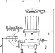
D2 D2 D C. W. L.: Continuous Running Water Level L. W. L.: Lowest Running Water Level
