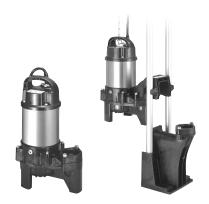
The PU-series is a submersible portable vortex pump designed for raw sewage, wastewater, and liquid carrying solid matters. It is made of resin and 304 stainless steel and excellent in corrosion-resistance. The vortex mechanism provides practically unchokable operation in sewage pumping. Liquid paraffin is used for the lubricating oil, which widens the application of the pump to decorative waterfalls, fishponds, aquaculture, etc.
