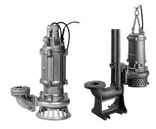
The SFQ-series is a submersible stainless steel casting high head corrosion-resistant pump designed for handling aggressive and corrosive liquids. The all wetted parts are made of 316 stainless steel, enables it to withstand demanding conditions found in construction, aggregate and mining applications. The pump with 5.5kW and above motor incorporates seal pressure relief port that prevents the pumping pressure from applying to the shaft seal.
