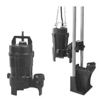
The UT-series is an economical type submersible vortex pump designed for handling raw sewage and wastewater from domestic and commercial areas. Rotation of the impeller produces vortex flow in the pump casing, which allows solid matters and fibrous materials to be pumped out with minimum contact to the impeller. Since this mechanism does not require those solid matters to pass through the impeller vane, the pump offers practically unchokable pumping.
