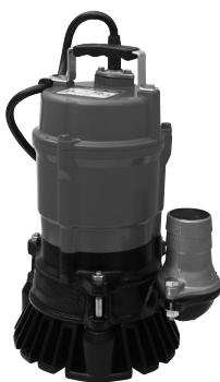
The HS-series is a submersible single-phase portable drainage pump. Though it is a single-phase unit, the pump has the durability equivalent to three-phase drainage pumps, since the wear parts are made of abrasion-resistant materials. The side discharge, spiral design allows smoother passage of the sucked solid matters. The shaft-mounted agitator prevents the air lock that tends to take place on vortex or semi-vortex pumps.
